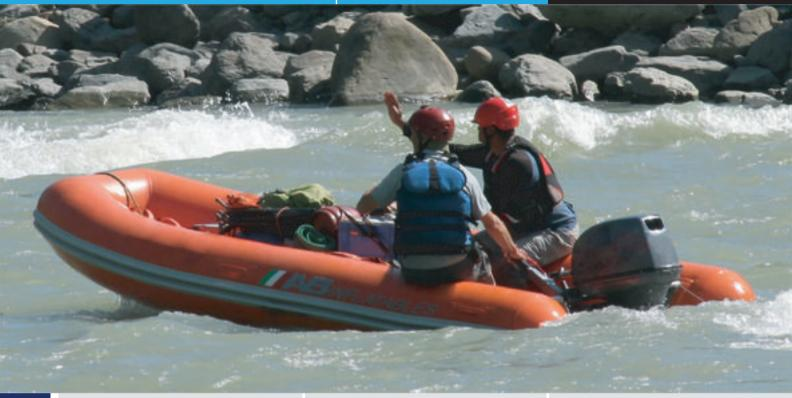
ے S **Overal Length** : 16'/ 4.88m **Number of Chambers** Shaft Length : 20" / 50.8cm : 10 **Overal Beam** : 7'/ 2.14m **Person Capacity** RDC Design Category : C Inside Length : 12'8"/3.85m Weight : 438lb/199kg Inside Beam : 3'6"/ 1.08m Recommended HP : 50hp/37.3kw Maximum HP Tube Diameter : 21"/ 0.53m : 60hp / 44.8kw
