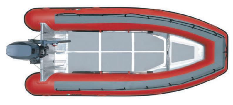
Overal Length : 13'/ 3.96m Number of Chambers : 3 Shaft Length : 20" / 50.8cm **Person Capacity Overal Beam** 6'5"/ 1.96m RDC Design Category : C Inside Length : 9'10"/3.00m Weight : 282lb/128kg Inside Beam : 3'3"/ 0.99m Recommended HP : 30hp /22.4kw Maximum HP Tube Diameter : 18"/ 0.46m : 40hp / 29.8kw
