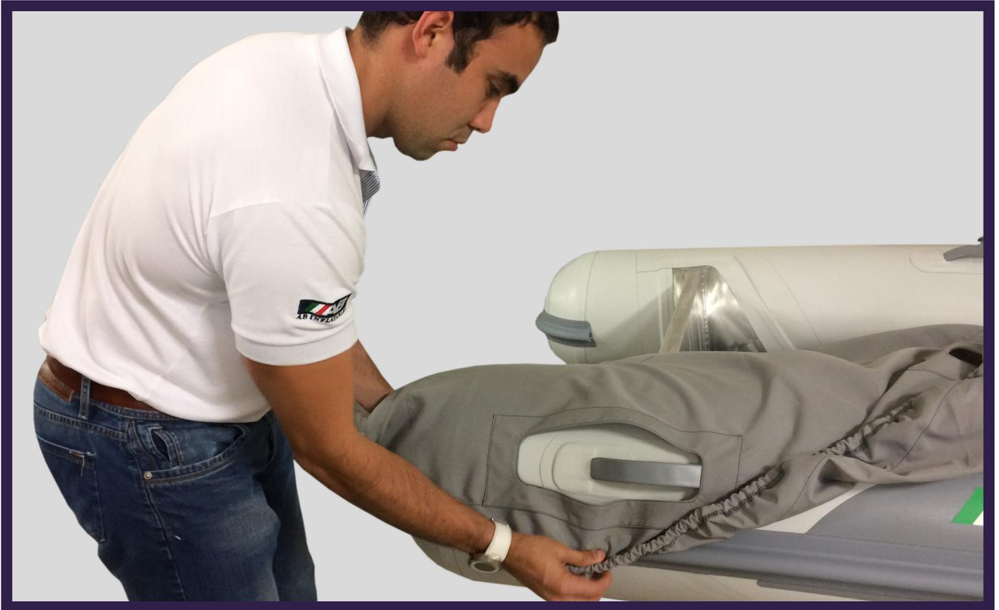
**Start from one of the dinghy cones adjusting the fabric below the rub rail.**
