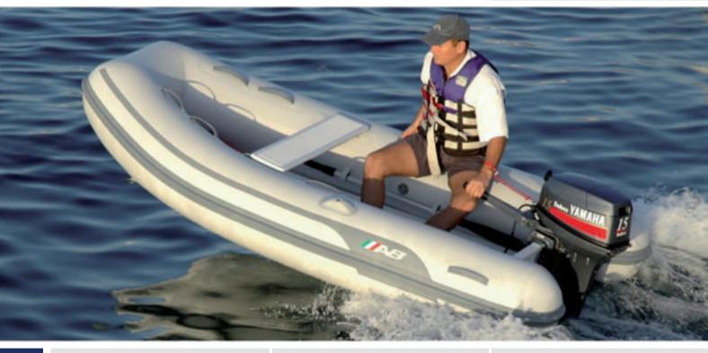
ے S **Overal Length** : 9'1"/ 2.76m **Number of Chambers** Shaft Length : 15" / 38.1cm **Overal Beam Person Capacity** : 4 : 4'9"/ 1.45m RDC Design Category : C Inside Length : 6'3"/ 1.90m Weight : 79lb / 36kg Inside Beam : 2'2"/ 0.66m Recommended HP : 8hp / 6.0kw Tube Diameter : 16"/ 0.40m Maximum HP : 10hp / 7.5kw
