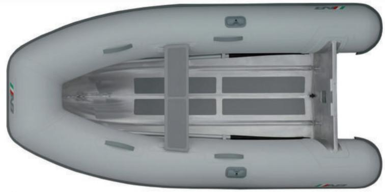
Overal Length : 8'5"/2.56m Number of Chambers : 2 Shaft Length : 15" / 38.1cm **Person Capacity Overal Beam** : 4'11"/ 1.50m RDC Design Category : C Inside Length : 5'10"/ 1.79m Weight : 68lb/31kg Recommended HP Inside Beam : 2'2"/ 0.66m : 4hp/3.0kw **Tube Diameter** : 16"/ 0.40m Maximum HP : 5hp/3.8kw
