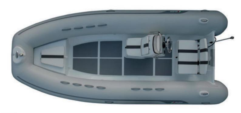
**Overal Length** : 16′/ 4.88m Number of Chambers : 5 Shaft Length : 20" / 50.8cm **Overal Beam Person Capacity** : 10 RDC Design Category : C : 7'/ 2.14m
