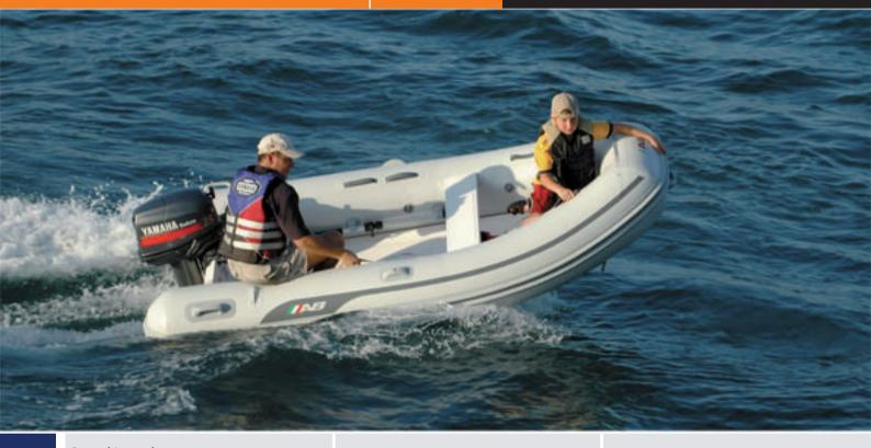
**Overal Length** : 10'6"/3.19m Number of Chambers : 3 + 1Shaft Length : 15" / 38.1cm **Overal Beam Person Capacity** : 5 RDC Design Category : C : 5'7"/1.72m
